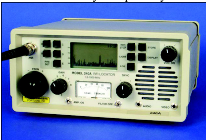
Fig. 4. The Radar Engineers Model 240 HF-UHF RFI Locator is a professional-grade receiver for locating RFI sources. It has a built-in oscilloscope display for recording and observing noise signatures. This receiver operates from 1.8 to 1000 MHz.
