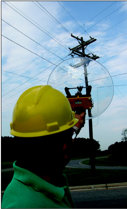
Fig. 8. The Radar Engineers Model 250 Parabolic Pinpointer is used to find an RFI source on a utility pole. The clear-plastic parabola is an "ear" connected to an ultrasonic detector that lets utility personnel listen to a power-line arc.
